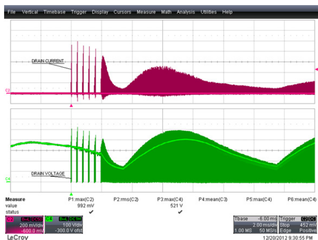
Figure 39 – 265 VAC, 50 Hz Start-up. Upper: I_{DRAIN} , 200 mA / div. Lower: V_{DRAIN} , 100 V, 2 ms / div.
