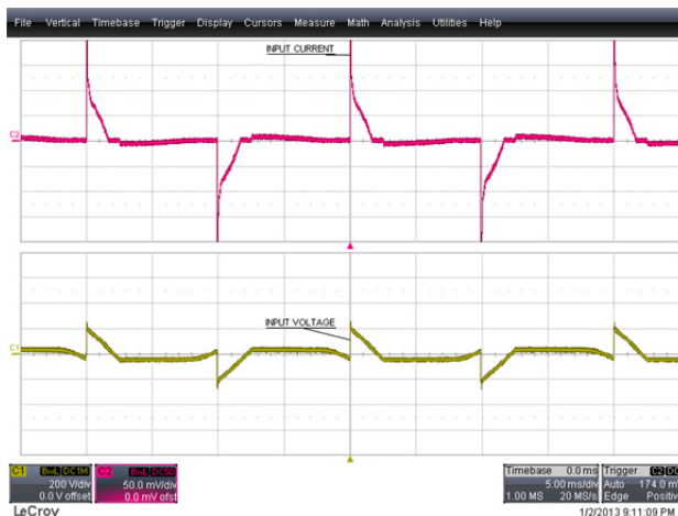
Figure 60 – 45° Conduction Angle. Upper: I_{IN} , 50 mA / div. Lower: V_{IN} , 200 V, 5 ms / div.
