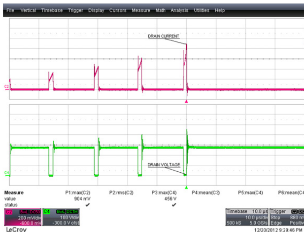
Figure 38 – 190 VAC, 50 Hz Start-up. Upper: I_{DRAIN} , 200 mA / div. Lower: V_{DRAIN} , 100 V, 10 \mu s / div.
