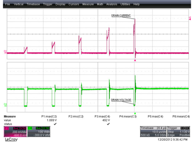
Figure 42 – 190 VAC, 50 Hz Output Short Condition. Upper: I_{DRAIN} , 200 mA / div. Lower: V_{DRAIN} , 100 V, 10 \mu s / div.
