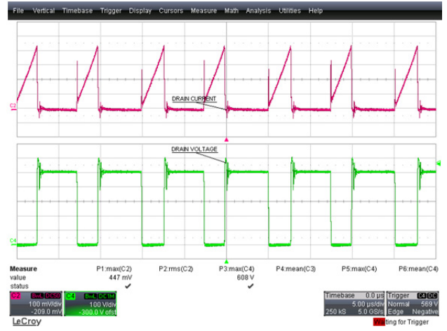
Figure 36 – 265 VAC, 50 Hz. Upper: I_{DRAIN} , 100 mA / div. Lower: V_{DRAIN} , 100 V / div., 5 \mu s / div.
