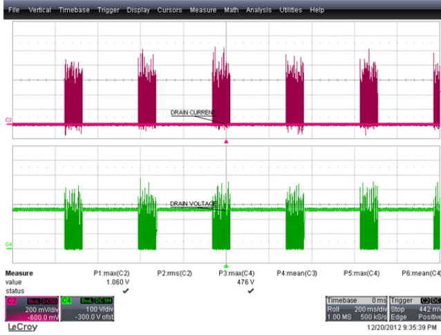
Figure 41 – 190 VAC, 50 Hz Output Short Condition. Upper: I_{DRAIN} , 200 mA / div. Lower: V_{DRAIN} , 100 V, 200 ms / div.
