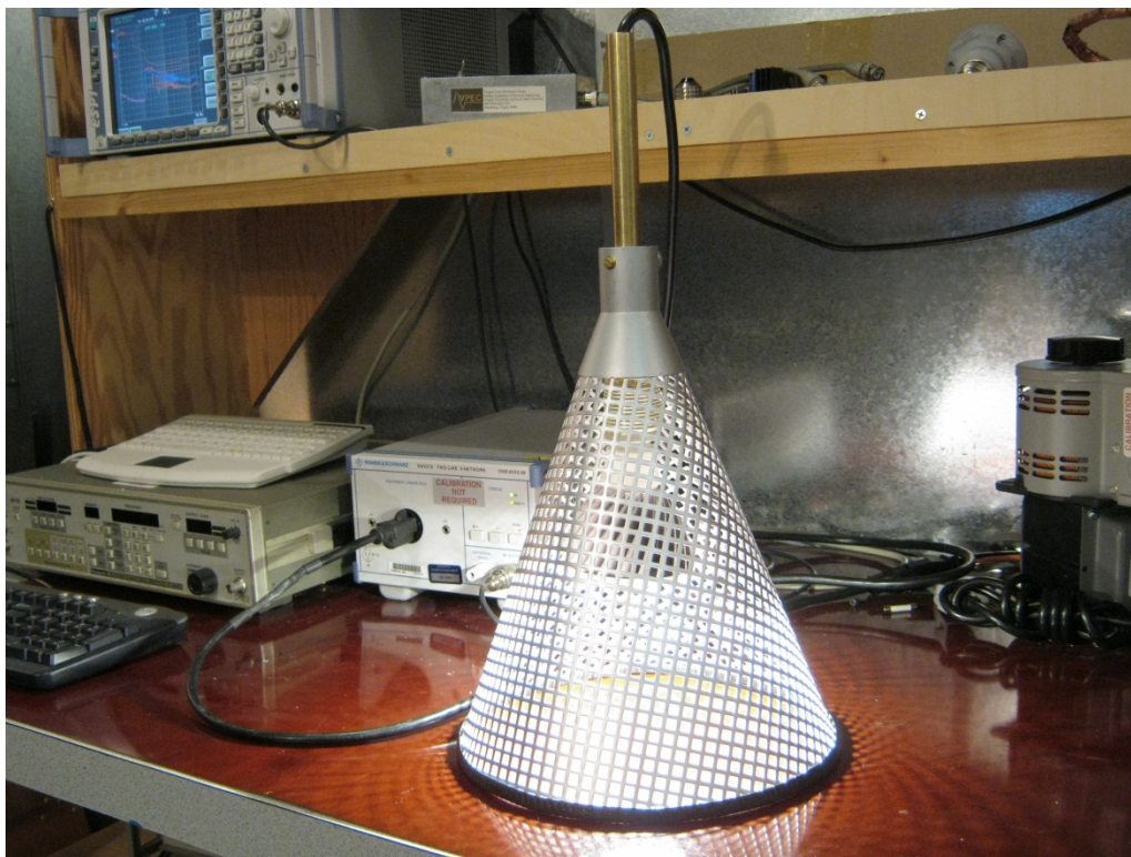
Figure 65 – EMI Test Set-up with the Unit and LED Load Placed Inside the Cone.
