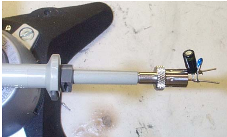
Figure 13 - Oscilloscope Probe with Probe Master 5125BA BNC Adapter (Modified with wires for probe ground for ripple measurement, and two parallel decoupling capacitors added).
