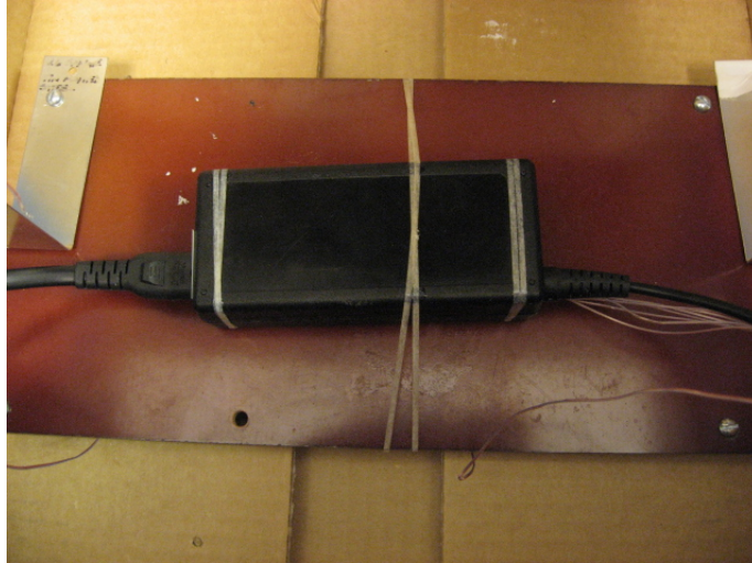
Figure 26 – Unit Inside the Box to Avoid Chamber Fan Influence.
