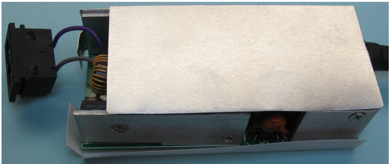
Figure 2 – Assembly Unit with Heat Spreader.
