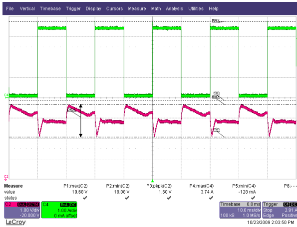
Figure 44 – Transient Response, 90 VAC, 0.1 A - 3.4 A - 0.1 A Load Step. Upper: Load Current, 1 A / div. Lower: V_{\text{OUT}} , 1 V / div. Time Scale: 10 ms / div.
