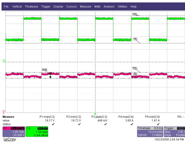
Figure 46 – Transient Response, 90 VAC, 50-100-50% Load Step. Upper: Load Current, 1 A / div. Lower: V_{\text{OUT}} , 1 V / div. Time Scale: 10 ms / div.
