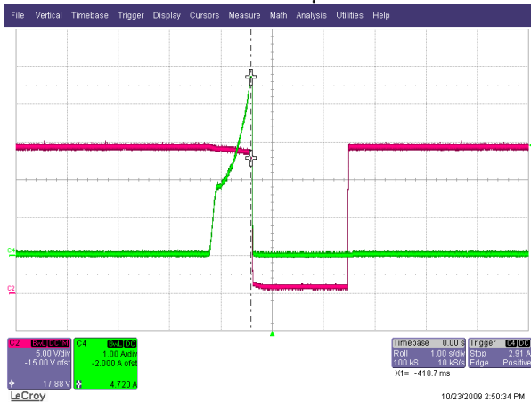
Figure 38 – 115 VAC, OCP Auto Recovery. Upper: I OUT , 1 A / div. Lower: V OUT , 5 V / div.
