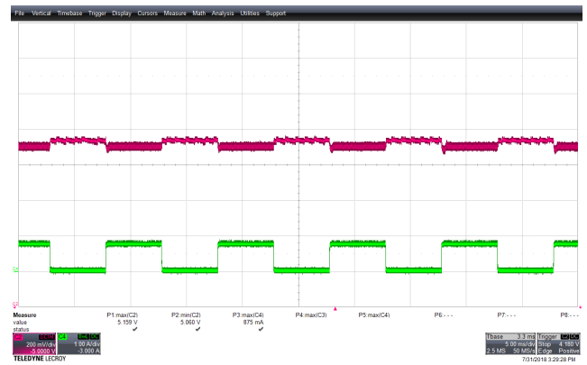
Figure 53 – Transient Response. 265 VAC, 5.0 V, 0 – 0.75 A Load Step. V_{MIN} : 5.060 V, V_{MAX} : 5.159 V. Upper: V_{OUT} , 0.2 V / div., 5 ms / div. Lower: I_{LOAD} , 1 A / div.
