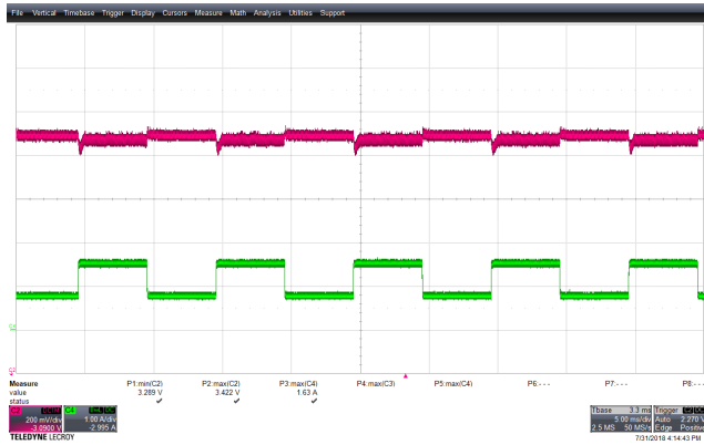
Figure 78 – Transient Response. 85 VAC, 3.3 V, 0.75 – 1.5 A Load Step. V_{MIN} : 3.289 V, V_{MAX} : 3.422 V. Upper: V_{OUT} , 0.2 V / div., 5 ms / div. Lower: I_{LOAD} , 1 A / div.
