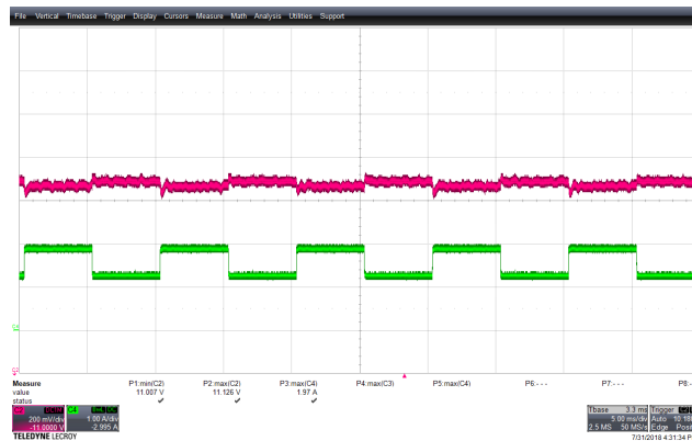
Figure 73 – Transient Response. 265 VAC, 11 V, 1.22 – 1.835 A Load Step. V_{MIN} : 11.007 V, V_{MAX} : 11.126 V. Upper: V_{OUT} , 0.2 V / div., 5 ms / div. Lower: I_{LOAD} , 1 A / div.
