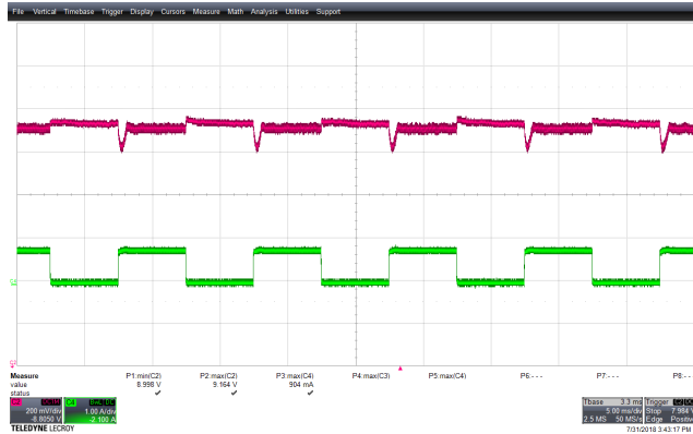
Figure 60 – Transient Response. 85 VAC, 9.0 V, 0 – 0.75 A Load Step. V MIN : 8.998 V, V MAX : 9.164 V. Upper: V OUT , 0.2 V / div., 5 ms / div. Lower: I LOAD , 1 A / div.
