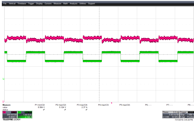
Figure 64 – Transient Response. 85 VAC, 9.0 V, 1.5 – 2.25 A Load Step. V_{MIN} : 8.984 V, V_{MAX} : 9.124 V. Upper: V_{OUT} , 0.2 V / div., 5 ms / div. Lower: I_{LOAD} , 1 A / div.
