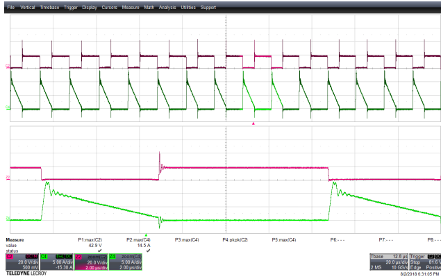
Figure 96 – SR FET Voltage Waveforms. 85 VAC, 11.0 V, 2.45 A Load (42.9 V MAX ). Upper: V DRAIN , 20 V, 20 μs / div. Lower: I DRAIN , 5 A / div. Zoom: 2 μs / div.
