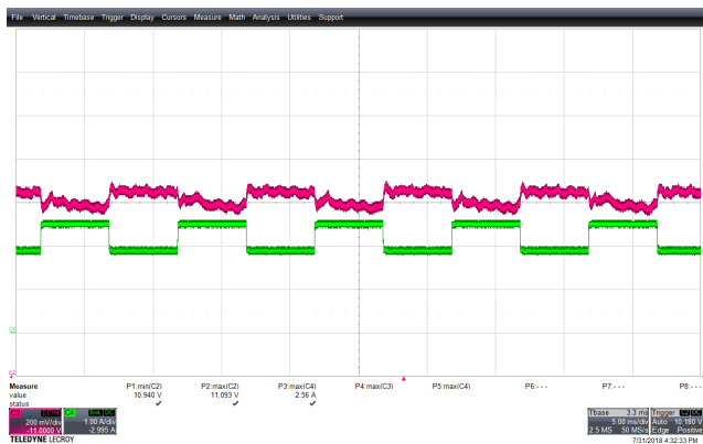
Figure 74 – Transient Response. 85 VAC, 11 V, 1.835 – 2.45 A Load Step. V_{MIN} : 10.940 V, V_{MAX} : 11.093 V. Upper: V_{OUT} , 0.2 V / div., 5 ms / div. Lower: I_{LOAD} , 1 A / div.
