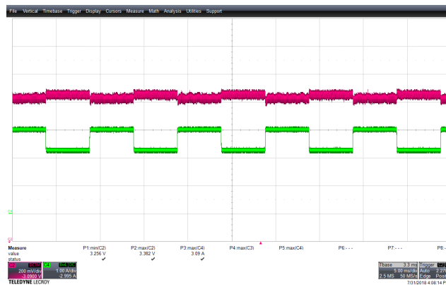
Figure 83 – Transient Response. 265 VAC, 3.3 V, 2.25 – 3 A Load Step. V_{MIN} : 3.256 V, V_{MAX} : 3.382 V. Upper: V_{OUT} , 0.2 V / div., 50 ms / div. Lower: I_{LOAD} , 2 A / div.
