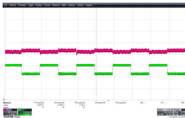
Figure 59 – Transient Response. 265 VAC, 5.0 V, 2.25 – 3 A Load Step. V_{MIN} : 4.973 V, V_{MAX} : 5.100 V. Upper: V_{OUT} , 0.2 V / div., 5 ms / div. Lower: I_{LOAD} , 1 A / div.
