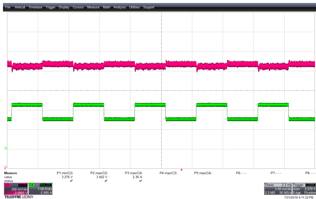
Figure 80 – Transient Response. 85 VAC, 3.3 V, 1.5 – 2.25 A Load Step. V_{MIN} : 3.276 V, V_{MAX} : 3.402 V. Upper: V_{OUT} , 0.2 V / div., 5 ms / div. Lower: I_{LOAD} , 1 A / div.
