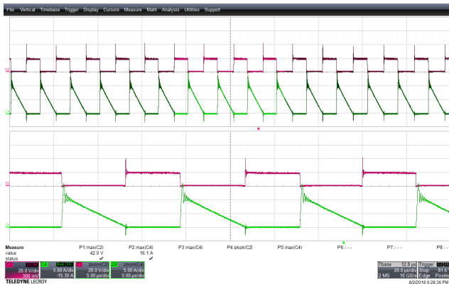
Figure 94 – SR FET Voltage Waveforms. 85 VAC, 9.0 V, 3 A Load (42 V MAX ). Upper: V DRAIN , 20 V, 20 μs / div. Lower: I DRAIN , 5 A / div. Zoom: 5 μs / div.
