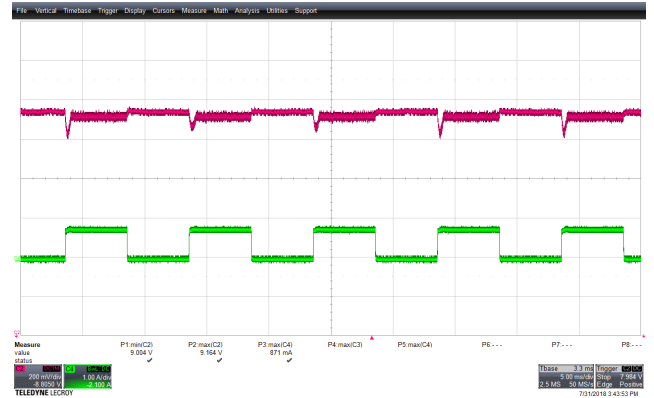
Figure 61 – Transient Response. 265 VAC, 9.0 V, 0 – 0.75 A Load Step. V MIN 9.004 V, V MAX : 9.164 V. Upper: V OUT , 0.2 V / div., 5 ms / div. Lower: I LOAD , 1 A / div.
