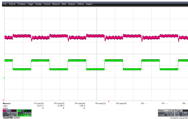
Figure 62 – Transient Response. 85 VAC, 9.0 V, 0.75 – 1.5 A Load Step. V MIN : 9.011 V, V MAX : 9.150 V. Upper: V OUT , 0.2 V / div., 5 ms / div. Lower: I LOAD , 1 A / div.
