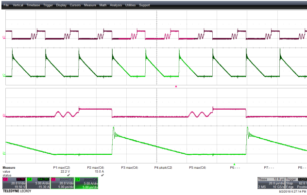
Figure 92 – SR FET Voltage Waveforms. 85 VAC, 5.0 V, 3 A Load (22.2 V MAX ). Upper: V DRAIN , 20 V, 20 μs / div. Lower: I DRAIN , 5 A / div. Zoom: 5 μs / div.
