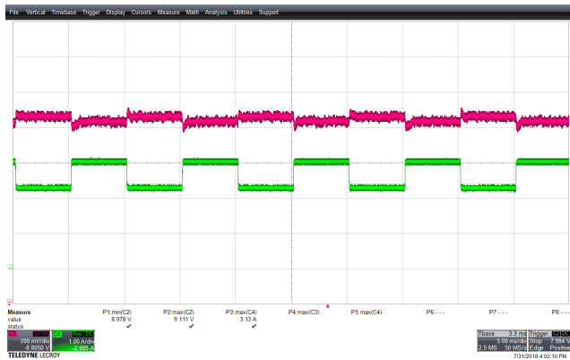
Figure 66 – Transient Response. 85 VAC, 9.0 V, 2.25 – 3 A Load Step. V_{MIN} : 8.978 V, V_{MAX} : 9.111 V. Upper: V_{OUT} , 0.2 V / div., 5 ms / div. Lower: I_{LOAD} , 1 A / div.
