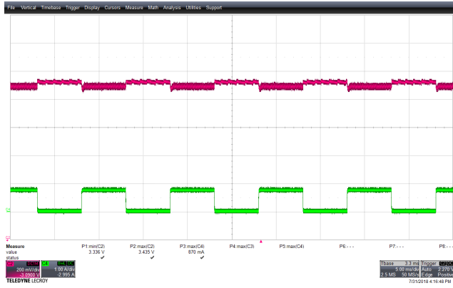
Figure 76 – Transient Response. 85 VAC, 3.3 V, 0 – 0.75 A Load Step. V_{MIN} : 3.336 V, V_{MAX} : 3.435 V. Upper: V_{OUT} , 0.2 V / div., 5 ms / div. Lower: I_{LOAD} , 1 A / div.
