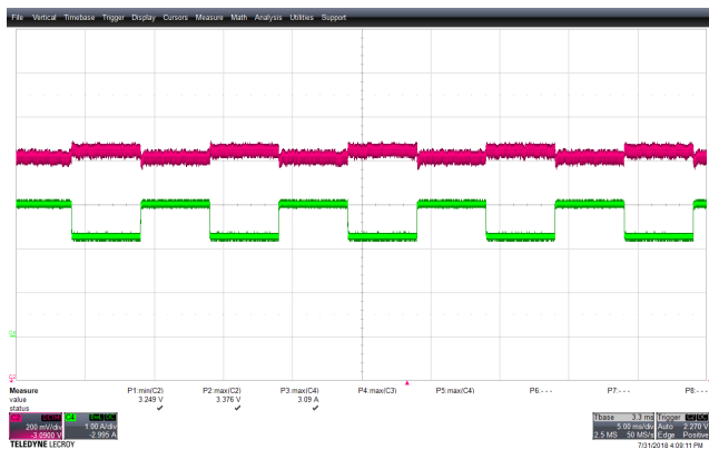
Figure 82 – Transient Response. 85 VAC, 3.3 V, 2.25 – 3 A Load Step. V_{MIN} : 3.249 V, V_{MAX} : 3.376 V. Upper: V_{OUT} , 0.2 V / div., 5 ms / div. Lower: I_{LOAD} , 1 A / div.
