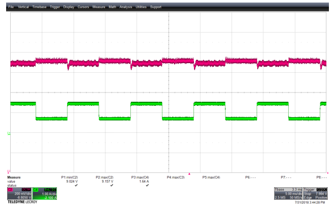
Figure 63 – Transient Response. 265 VAC, 9.0 V, 0.75 – 1.5 A Load Step. V MIN : 9.024 V, V MAX : 9.157 V. Upper: V OUT , 0.2 V / div., 5 ms / div. Lower: I LOAD , 1 A / div.
